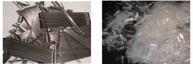
Fig. 1 Steel Fiber with Hooked-end and Polypropylene Fiber
